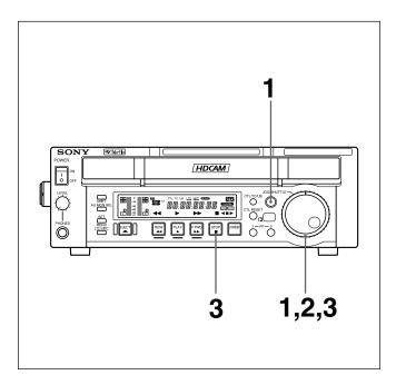
In shuttle mode, the SHUTTLE dial controls the playback speed based on the angular position of the dial. There are seven playback speeds:  $\pm 0.03$  times,  $\pm 0.12$  times,  $\pm 0.5$  times,  $\pm 1$  times,  $\pm 2$  times,  $\pm 2$  times.
